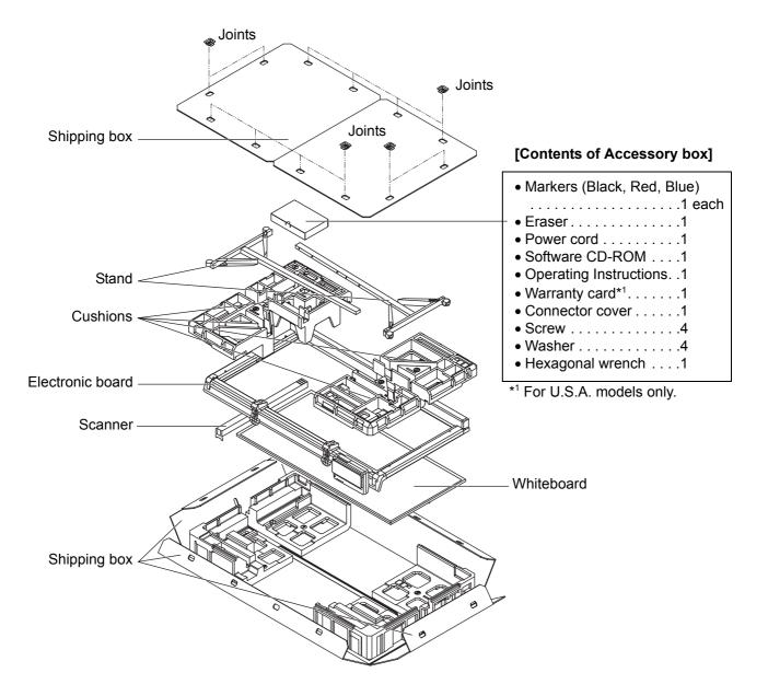
\* This is a diagram of the UB-2815C. UB-2315C is equipped with one board stopper and one board stopper lever.
