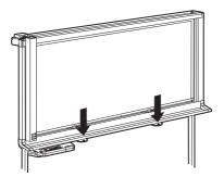
• Once the board stoppers are unlocked, it is possible to rotate the whiteboard.
